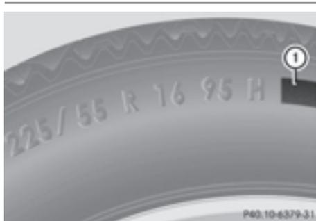
In addition to the load bearing index, load index ① may be imprinted after the letters that identify speed index ⑥ on the sidewall of the tire (▷ page 346).
