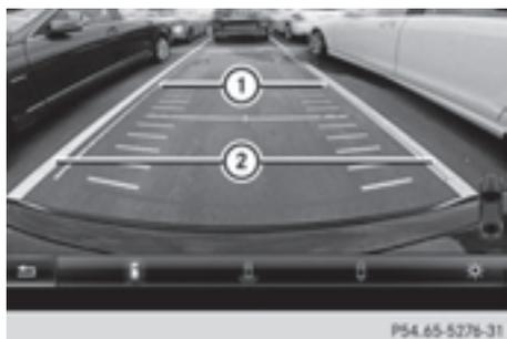
① White guide line at current steering wheel angle
