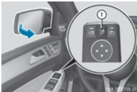
If you have switched the **Auto. Mirror Folding** on and you fold the exterior mirrors in using button ①, they will not fold out automatically (▷ page 105).
