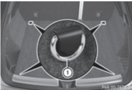
There are four cargo tie-down rings ① in the cargo compartment.
