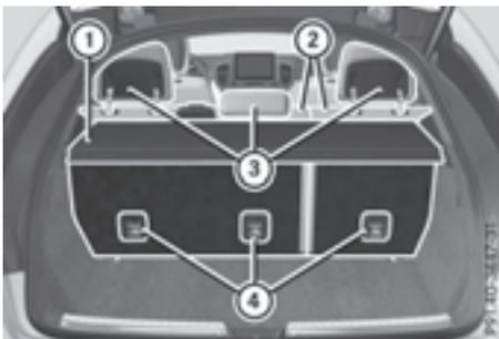
Top Tether anchorage points ④ are located on the rear side of the rear seat backrests.
