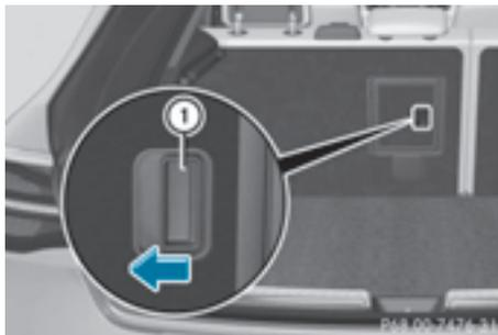
The through-loading facility is opened from the cargo compartment.
