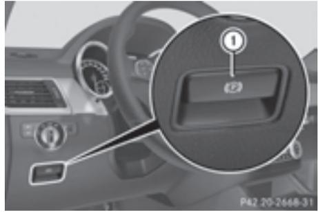
The vehicle can also be braked during an emergency by using the electric parking brake.
