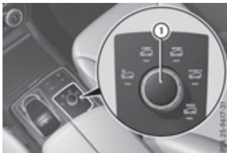
In the **Comfort** drive program, the driving characteristics of your vehicle are more comfortable. Therefore, select this mode if you favor a more comfortable driving style. Also select the **Comfort** drive program when driving fast on straight roads, e.g. on straight stretches of highway.
