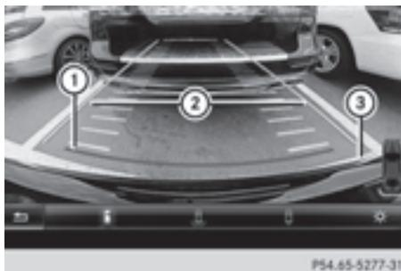
① Red guide line at a distance of approximately 12 in (0.30 m) from the rear of the vehicle
