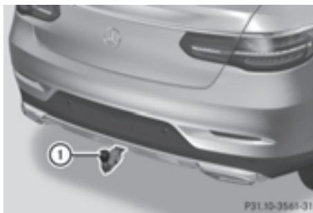
The ball coupling must be cleaned if it becomes dirty or corroded.
