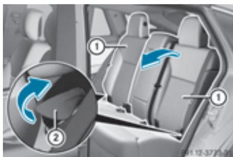
You can adjust the angle of the backrests in the second row of seats. There are several possible detent positions.
