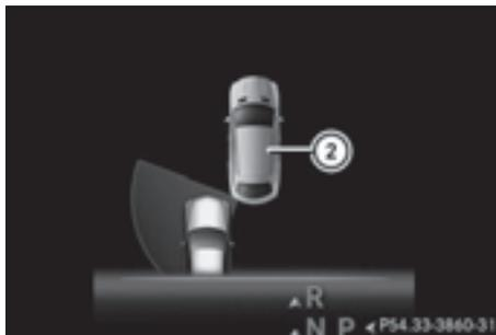
If a course-correcting brake application occurs, red warning lamp ① flashes in the exterior mirror and a dual warning tone sounds. In addition, display ② underlines the danger of a side collision appears in the multifunction display.
