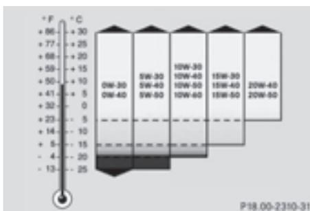
Viscosity describes the flow characteristics of a fluid. If an engine oil has a high viscosity, this
