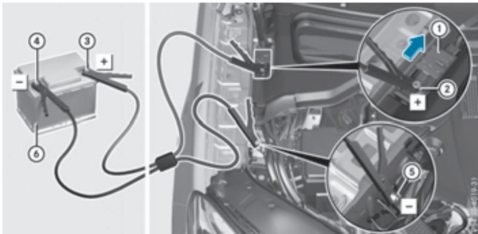
Position number ⑥ identifies the charged battery of the other vehicle or an equivalent jump-starting device.
