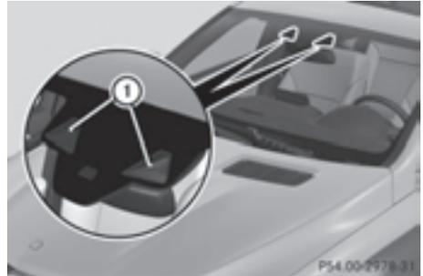
DISTRONIC PLUS with Steering Assist and Stop&Go Pilot aids you in keeping the vehicle in the center of the driving lane by means of moderate steering interventions at speeds of 0 - 125 mph (0 - 200 km/h).
