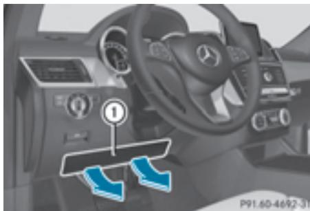
Driver's knee bag ① deploys under the steering column. The driver's knee bag is triggered together with the front air bag.
