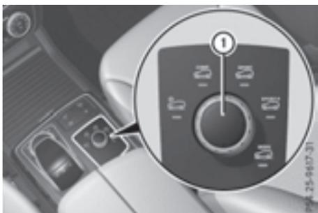
The very firm setting of the suspension setting in the **Sport Plus** drive program ensures the best possible contact with the road. Select this drive
