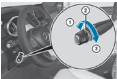
You can set the specified minimum distance for DISTRONIC PLUS by varying the time span between one and two seconds. With this function, you can set the minimum distance that DISTRONIC PLUS keeps to the vehicle in front, dependent on vehicle speed. You can see this distance in the multifunction display (▷ page 175).
