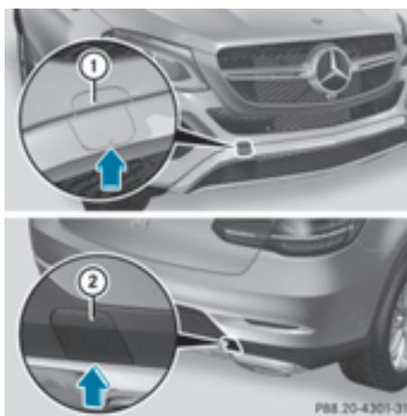
The brackets for the screw-in towing eye are located in the bumpers. They are at the front and rear behind covers ①②.
