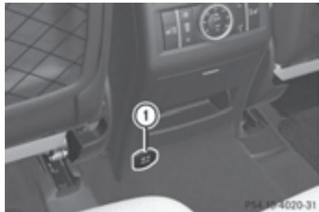
Vehicles with the Rear Seat Entertainment System have two sockets in the center console in the rear compartment.
