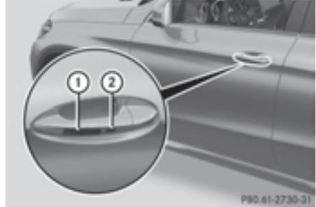
► **To unlock the vehicle:** touch the inner surface of the door handle.
