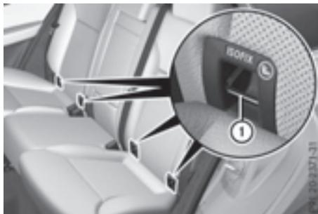
► Install the LATCH-type (ISOFIX) child restraint system on both LATCH-type (ISOFIX) securing rings ①.
