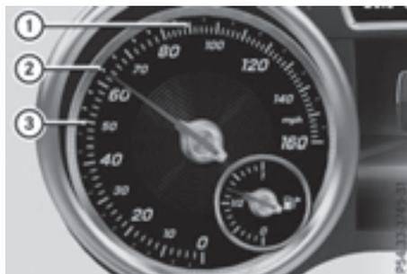
Example: DISTRONIC PLUS displays in the speedometer
